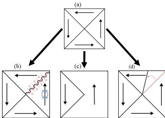
**Fig. 2.** Components of magneto-mechanical damping on the example of four  $90^\circ$  domains in a square cell of a ferromagnetic sample.
