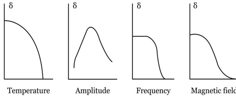
**Fig. 4.** Qualitative dependences of magneto-mechanical damping (MMD) on temperature, strain amplitude, loading frequency, and external magnetic field. Adapted from Ref. [25].
