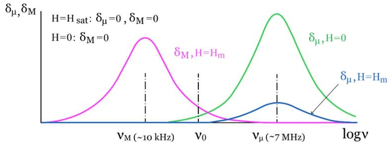
**Fig. 3.** Scheme of the influence of the frequency  $\nu$  on the components of the microeddy and macroeddy MMD with characteristic frequencies for  $\text{Ni}_2\text{MnGa}$ . Adapted from Ref. [24].
